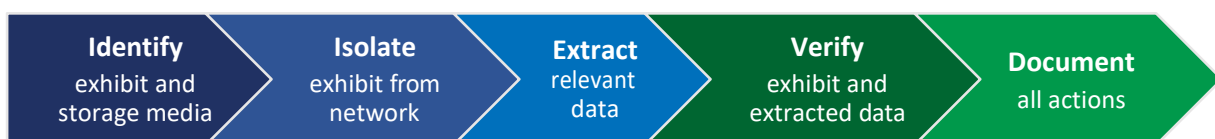
Figure 32: Extraction Process for Drones and Drone Remote Controllers
