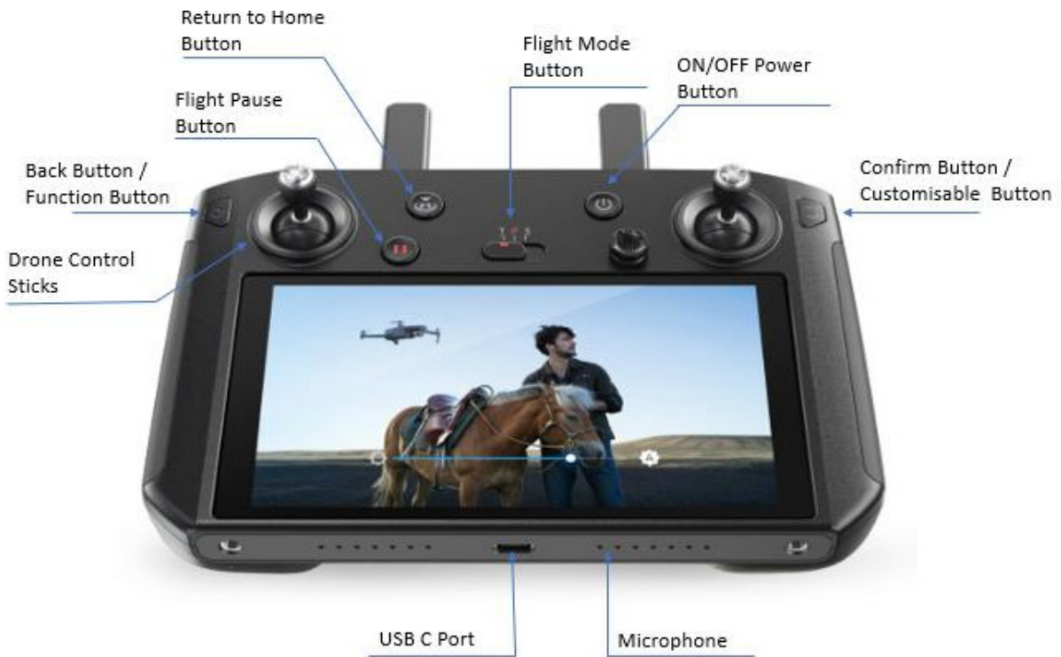
Figure 13: Integrated Drone Remote Controller
